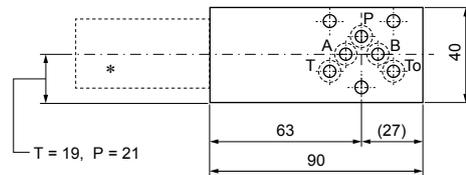
**Sandwich construction DN.SA04-A, B, AB**
