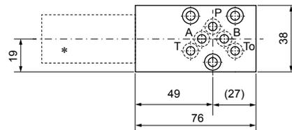
**Sandwich construction DN.SA04-P, T**
