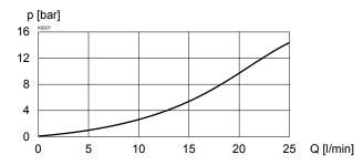
$\Delta p = f(Q)$  Pressure drop-volume flow curve 3-way operation
