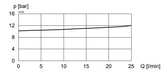
Q<sub>1</sub> = f (p) Leakage volume flow curve
