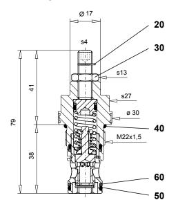
Cavity drawing according to ISO 7789–22–01–0–98
