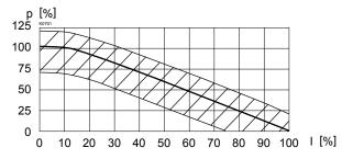
Adjustable range of nomial pressure, adjusted with set screw under the clamp cap.
