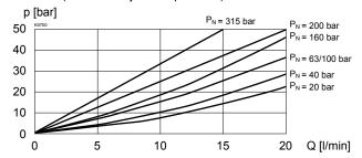
Q<sub>1</sub> = f (p) Leakage volume flow characteristics
