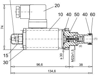
Cavity drawing according to ISO 7789–22–02–0–98
