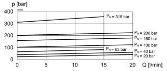
p = f (I) Pressure adjustment characteristics (Q = 1 l/min)
