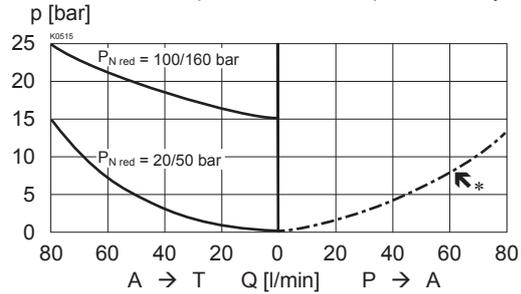
$p_{\text{red}} = f(n)$  Pressure adjustment characteristics
