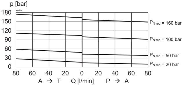
$p_{\text{red}} = f(Q)$  Pressure volume flow characteristics
