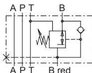
For sandwich red. pressure in B the adjusting parts are on A-side
