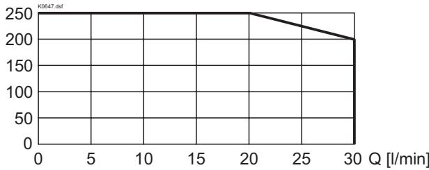
$\Delta p = f(Q)$  Pressure drop volume flow characteristics per control edge
