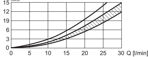
— Pressure drop for valves with no. 3 spool and flow P to T only.
