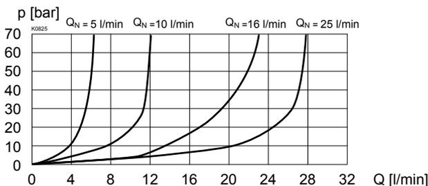
$\Delta p = f(Q)$  Pressure loss/flow characteristics ( $l = l_G$ )
