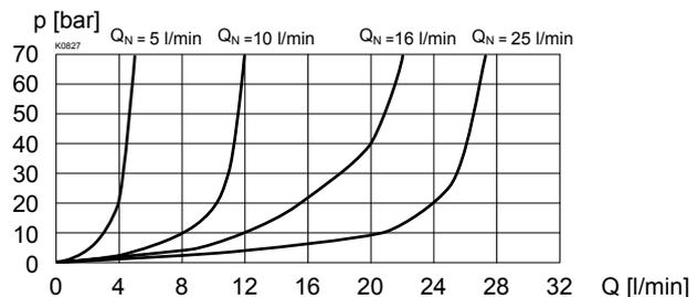
Q = f (l) Volume flow adjustment characteristics ( $\Delta p = 20 \text{ bar}$ )
