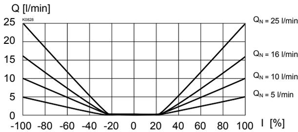
Q = f (l) Volume flow adjustment characteristics ( $\Delta p = 20 \text{ bar}$ )
