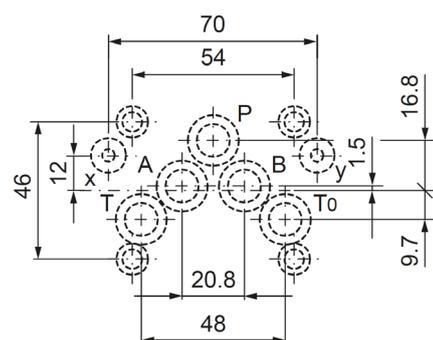
Raccordement hydraulique NG10
