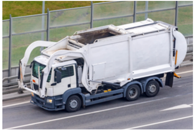
Front-loading refuse collecting vehicle in transport mode
