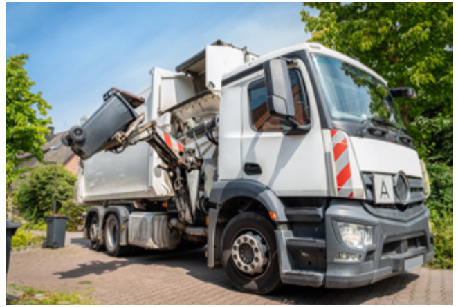
Side-loading bin , side-loading refuse collecting vehicle in operation
