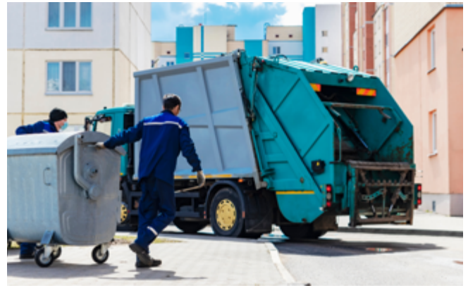
Rear-loading refuse collecting vehicle in action
