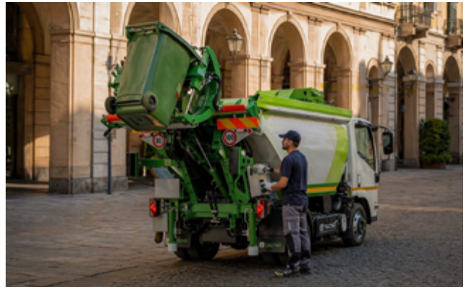
Mini rear-loading compact refuse collecting vehicle in action
