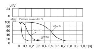
Schifting times, Influence of orifices on shifting Mesured with AMW4D61-G24, Q = 7 l/min Solenoid deenergised
