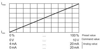
Operation mode: unipolar, 2-solenoid valve
