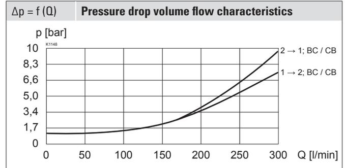
**Attention!** Measured with cavity according to data sheet 2.13-1059 (annular groove)
